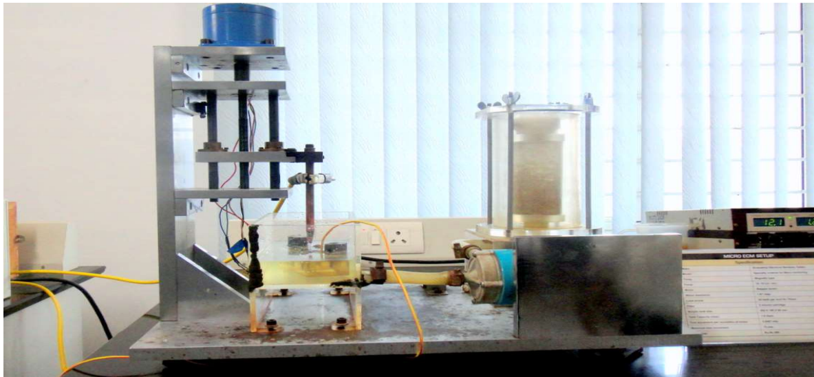
Fig:1 Machining set up of micro-ECM
