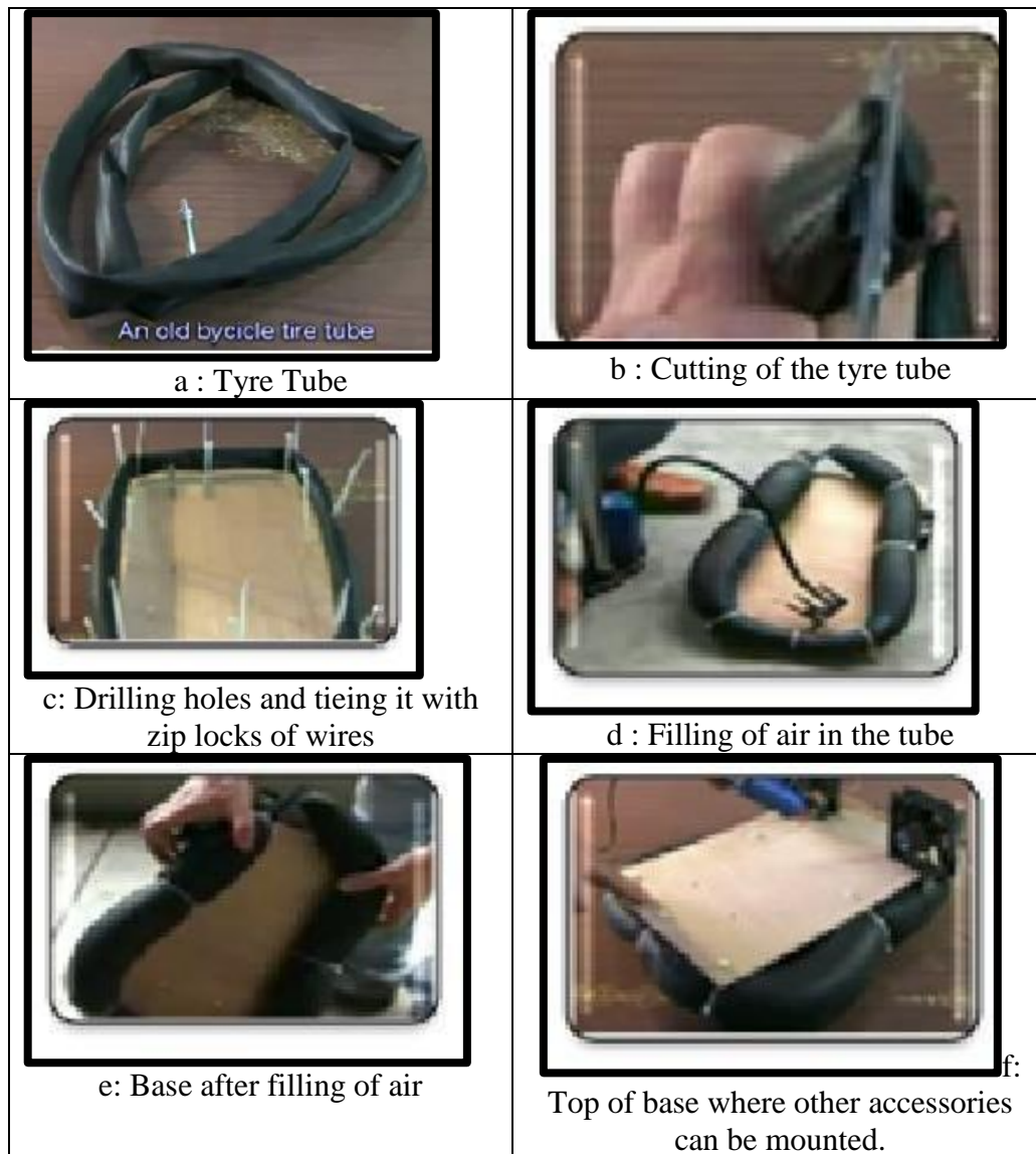
Figure 2 : Steps of base making
