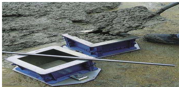
Fig. 1. Casting of Concrete Cubes (M25)
