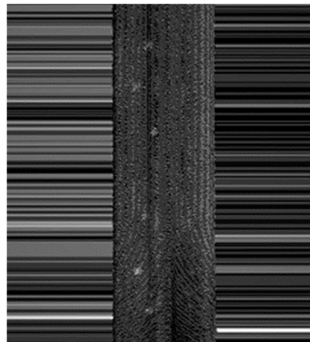
Fig. 3. An example of the edge differential image between inspected and master images.
