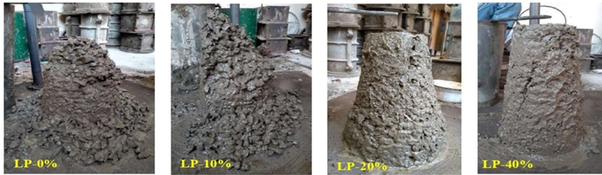
(i) Shear slump (ii) Collapse (iii) True slump (iv) True slump (a) Photograph showing the effect of limestone powder on the slump of concrete
