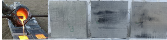
Fig. 6. Casting and specimen preparation process
