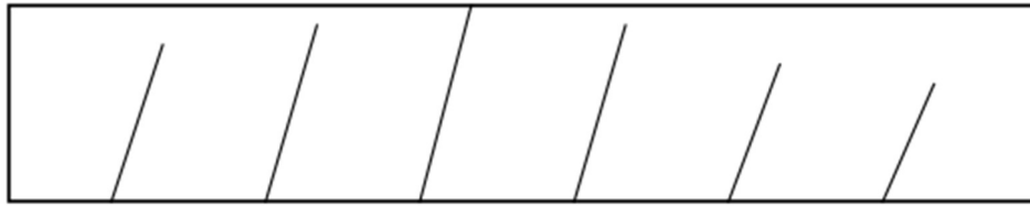
Fig. 3 Typical crack pattern and failure mode
