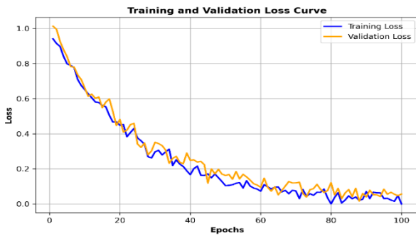
Fig.2(a) Training and validation loss and accuracy curve showing steady convergence and low overfitting across 100 epochs .
