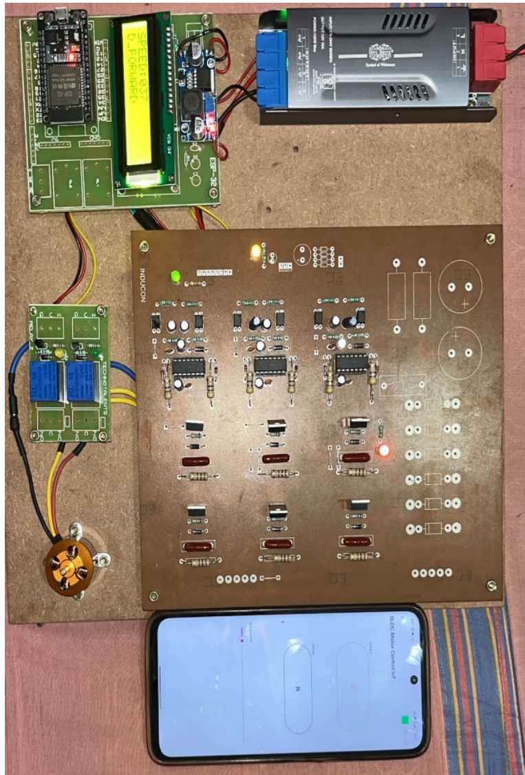
Fig. 4. Prototype with local display and wireless user interface.
