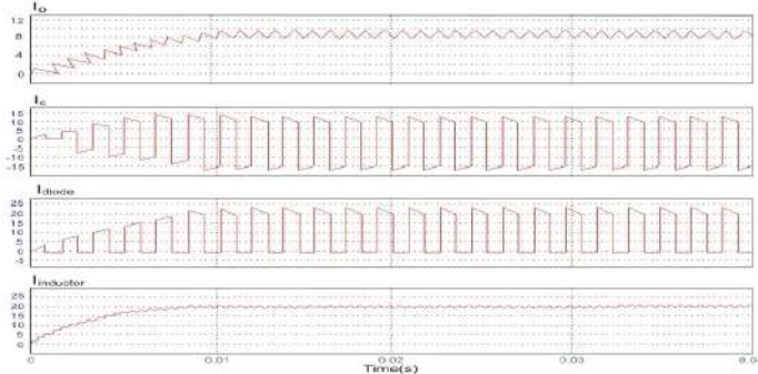
Figure:7- Simulation output waveforms of a DC–DC converter solar Electric-Vehicle charging / MPPT
